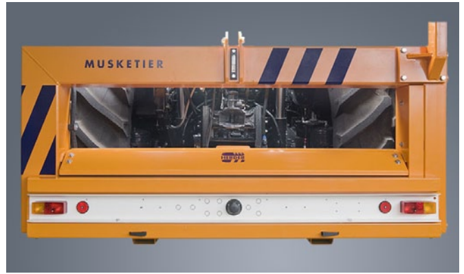
Special hydraulic tank at the rear ensures that the upper tow bar remains accessible for a trailer.
