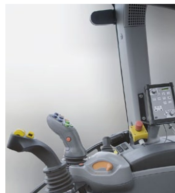
The joystick provides for a precise operating of the booms. During mowing, Nivotronic provides for the following of the terrain contour.
