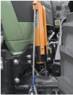
Stabilising cylinder for fixed front axle increases the stability.
