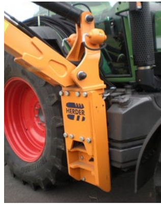
Pivot 'rotary cylinder' for smaller construction.
