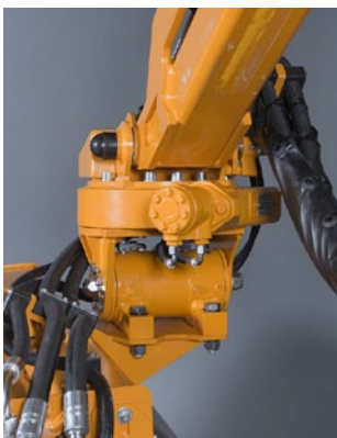
Stabilising cylinder for fixed front axle increases the stability.
